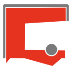
R0180 Radial shaft seal with spring dust lip
