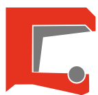
R0110 Radial shaft seal with spring and dust lip
