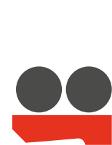
AB200 Double-acting wiper with supporting O-rings
