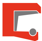
R0100 Radial shaft seal with spring
