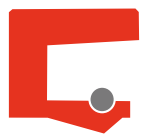
R0200 Radial shaft seal with spring
