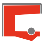
R0110 Radial shaft seal with spring and dust lip
