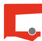
R0210 Radial shaft seal with spring and dust lip
