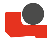
AB150 High-performance wiper with bevelled lip
