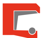
R0100 Radial shaft seal with spring
