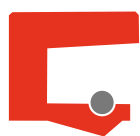
R0200 Radial shaft seal with spring
